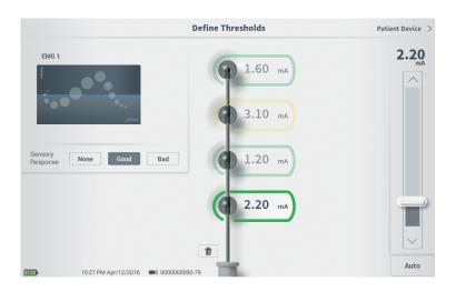
The thresholds saved to the Neurostimulator can be updated in the **Define Thresholds** screen. The screen displays the currently saved threshold data until test stimulation is delivered to set new thresholds. For more information on setting thresholds, see *Define Tined Lead Thresholds* in the *Test Stimulation During Lead Implantation* section of this manual.
