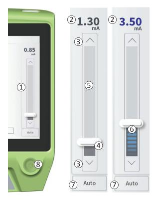
The stimulation bar (1) controls the stimulation amplitude during test stimulation for lead placement and Neurostimulator programming. When available, the stimulation bar is on the right side of the **CP** screen. The stimulation bar includes:
