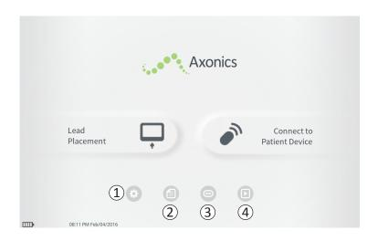
The **Home** screen will appear after successful log-in to the CP or after exiting any CP function (e.g., "Lead Placement"). The **Home** screen provides access to tools to assist in data management and the use of the CP, including:
