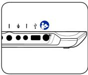
To charge the CP, plug the power supply into a power outlet and into the CP. The power supply plugs into the CP at the right end of the Connection Panel and is indicated by the "Refer to manual" symbol .
