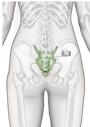
Figure 2-1: Axonics SNM System implant location eligible for MRI scan with Whole-Body RF transmit coil (Neurostimulator 1101 is shown as an example)
