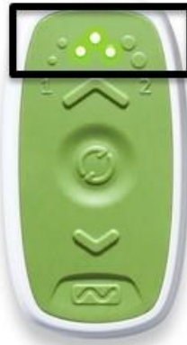
a. device is ready for whole-body MRI
