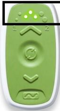
a. device is ready for whole-body MRI
