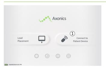
The CP can connect to a patient's external Axonics Trial Stimulator (Model 1601) or implanted Neurostimulator (Model 1101) to check the status of the device and program the device.
