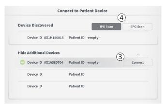
Additional devices can be displayed by the CP if the first device found is not the targeted Stimulator. Press the down arrow next to "Show Additional Devices" (1). This will display up to 3 additional devices found in proximity of the CP.
