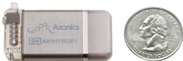
Figure 1. System includes rechargeable, miniaturized INS about 5 cc in volume with 15-year approved life in Europe, Canada and Australia.
